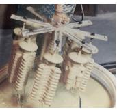
3. Control removal of soluble wax cores. When an acid leach is used to eliminate soluble wax, it should be properly rinsed to prevent acid from being carried over into the slurry; as this can cause slurry pH to drop and the slurry to gel.
